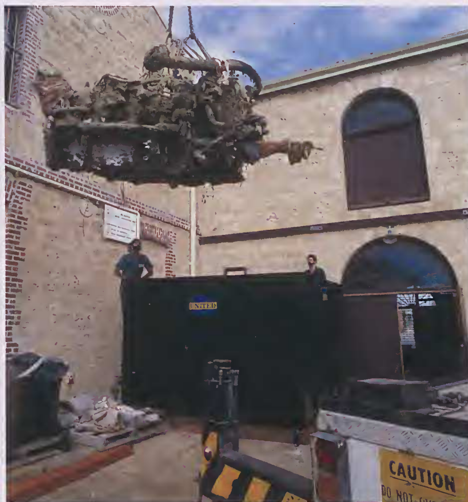
Figure 12 Xantho engine being loaded into conservation tank prior to treatment (WA Museum © photo BTA0708).
